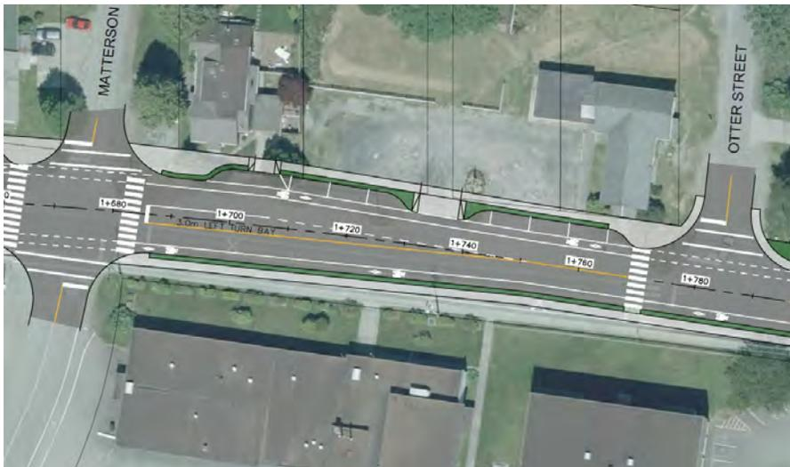
Remodeling Peninsula Road will allow for designated parking spaces, and a wider road width. Concept plans have been developed by McElhaney and presented to the District. This will include additional sidewalks, bike lanes and increased driving lanes. This design will not provide any additional safety measures but will
